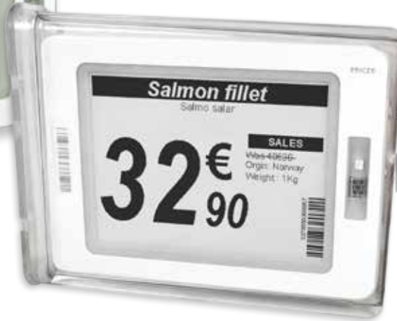
SmartTAG HD 110 with water protective box
